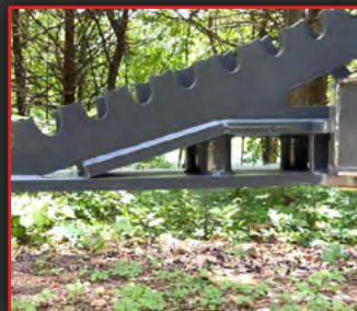
Gap Allows Dirt to Flow
