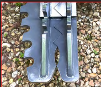
Opening for Post Pulling
